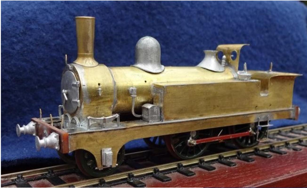
I am grateful to 5&9 Models for many of the castings and to various etched kit designers (in particular EBM and RT Models) both for useful pieces that were surplus to the original kit and for scrap etch in nice straight thin pieces. Never throw away bits of fret; you don't know when they will come in handy!
