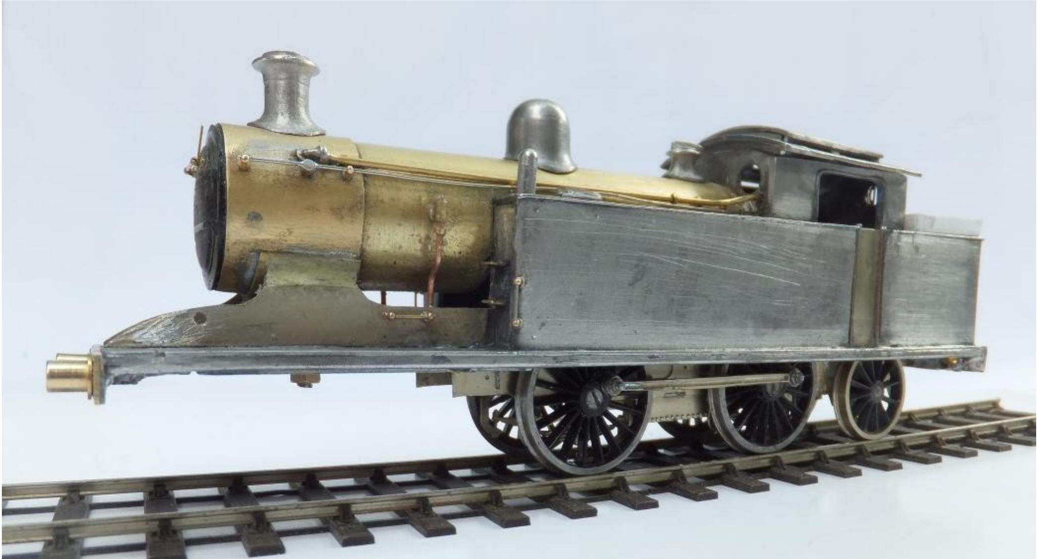
Boiler bands will be added after painting, but other detail such as lamp irons and steps, and under footplate features will be added after the chassis has been made, but as yet this has not been started but will follow a similar but not identical pattern to the I1x.
