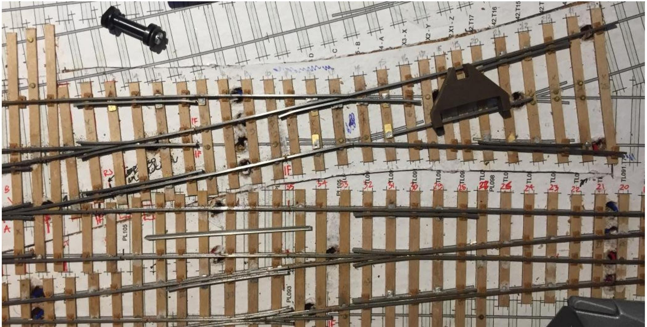
Figure 9 Progressing with the diamond. At least two flangeway gauges are desirable for getting the obtuse crossings right! Both roads are curved, so the common crossings are quite different – 1:8 at one end, and 1:3.4 at the other. The 1:8 is a C&L complete crossing, one of several purchased for such purposes. The big holes for the droppers weren't planned, it's just that I needed a drill bit long enough to clear two layers of ply, cork and pink foam, and the shortest available was 6mm diameter.
