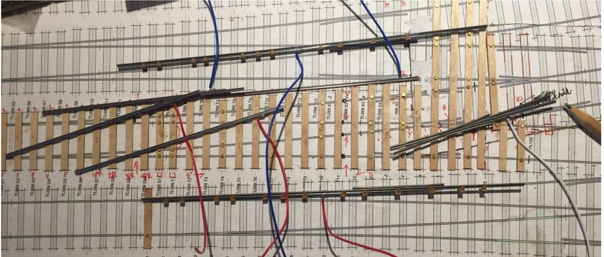
Figure 7 Rivetted timbers down for the first turnout, and P4 Track Company rail components prepared. Note that check rails are already in place against the stock rails, given that the kits include the check chairs. Dropper wires have already been soldered to the underside of the rail.
