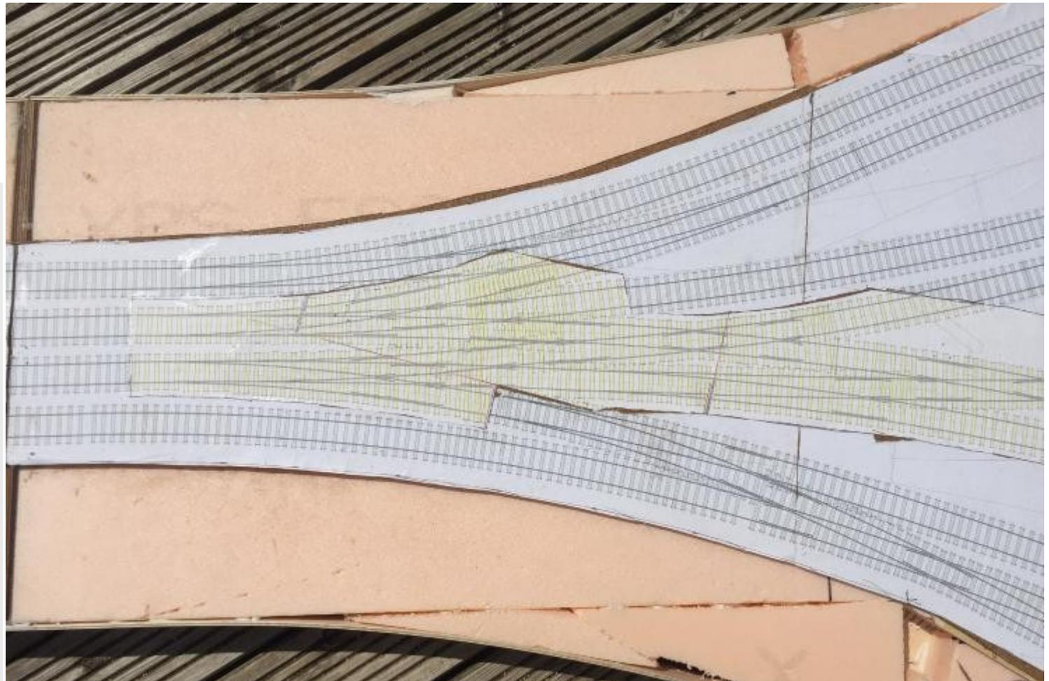
Figure 6 Scaled copy of the Network Rail roof plan positioned in the 'Y' of the station. This will be on a separate drop-in piece supported by ledges on the London and Brighton boards. The Brighton tracks (at least the double-faced one) will need to be slewed slightly to the left to match the roof plan – OS maps are good, and often all we have, but you can't expect them to be completely accurate.
