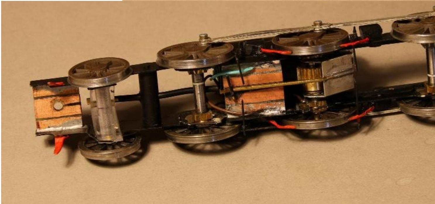
The loco is fully compensated with split axle pick-ups, Sharman wheels, Mashima motor and HighLevel gearbox. The radial axle box is made from Perspex.
