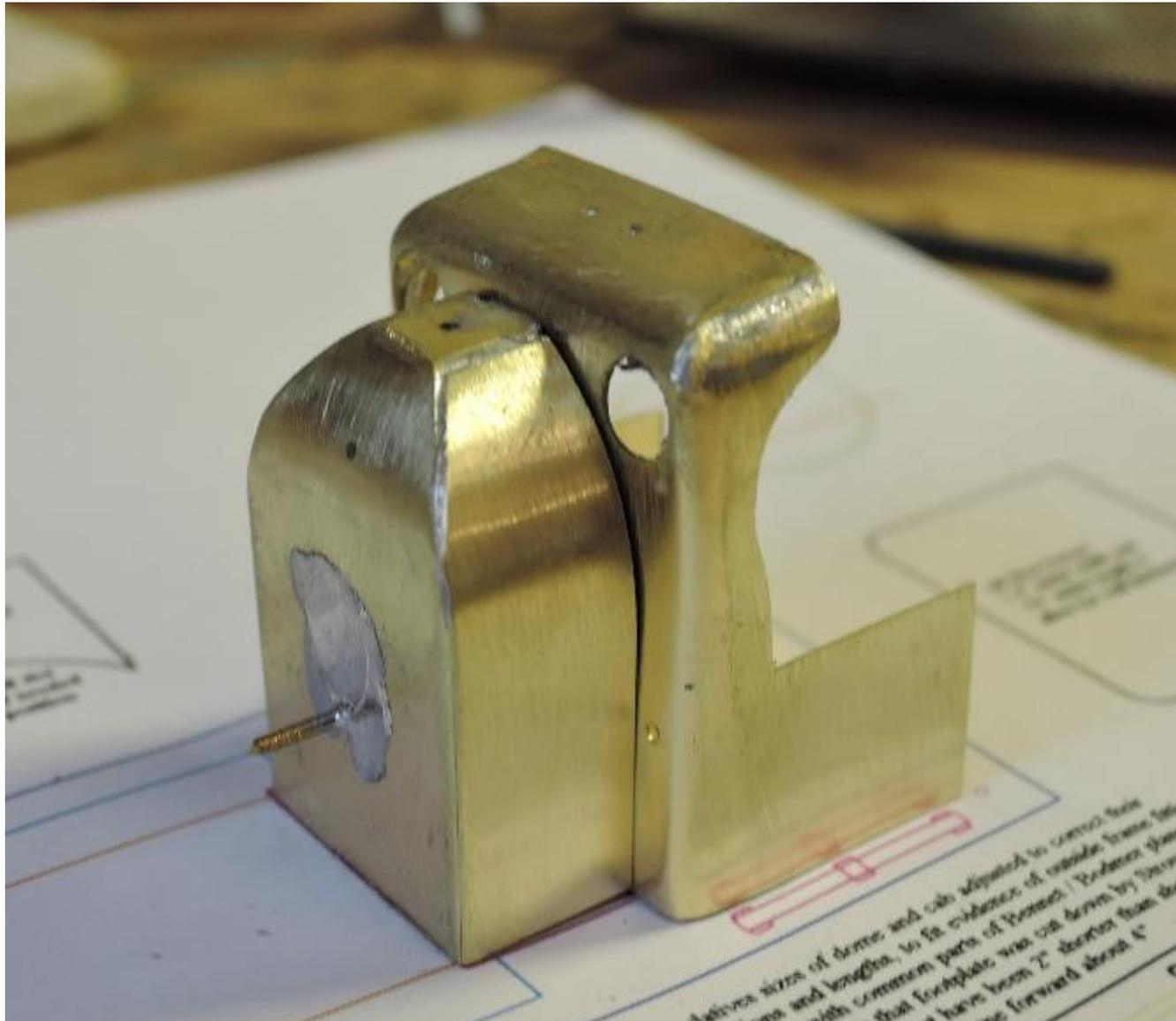
*Figure 3. The cab and Haycock firebox sections temporarily joined and tested against my cutting plans. The fold pattern of the cab created a small hole in each top corner that was easily filled with solder and filed to shape. The corners of the Haycock firebox were also filed to create a small radius curve to each edge.*
