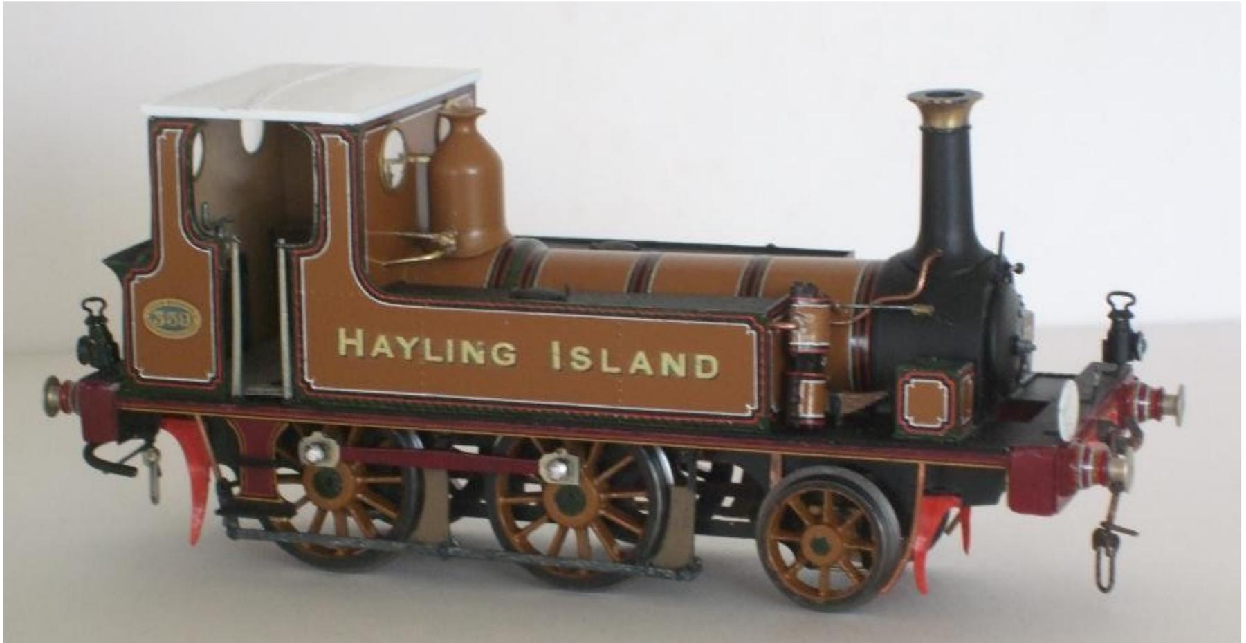
number of detailed photos of his superb model of "Inspector". In the absence of photographic evidence I am not sure if the pipes from the safety valve to the cab were a later addition to "Inspector". John Ritter suggested that Stroudley may well have fitted the improved Gifford injector manufactured by Gresham under license and that these pipes were the live steam supply. I couldn't use a spare Terrier cab roof, as it was too large, so filed one out of Plastikard.
