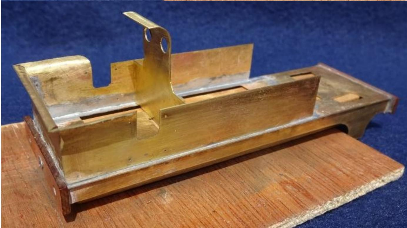
Side tanks/bunker sides now soldered – and the weatherboard plonked in place.
