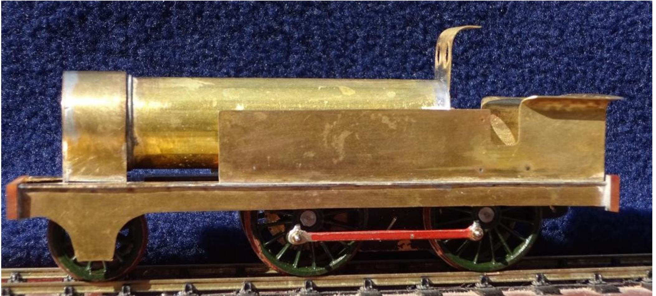
Sitting the boiler in place, coffee stirrers supported the boiler at the right height and helped to ensure an even gap between the boiler and the sidetanks on either side. Make sure that you pick up stirrers from a wide range of sources to maximise the range of thicknesses and widths!
