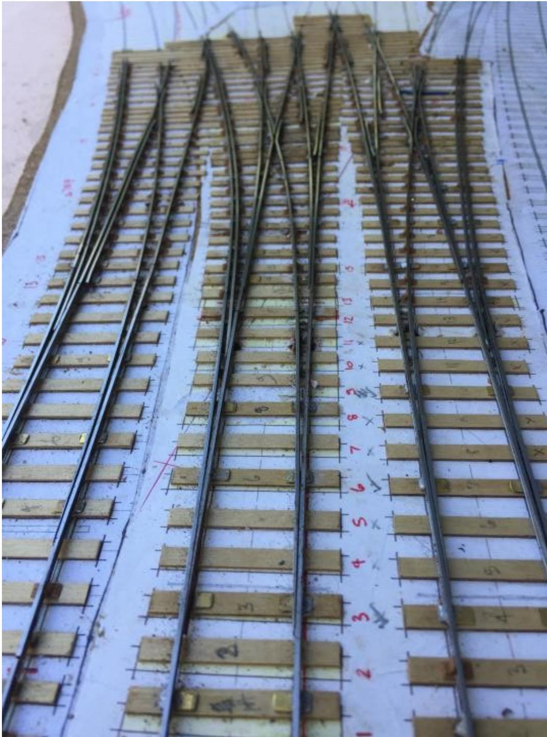
Figure 15 Second tandem added, also check railed on the right hand route.
