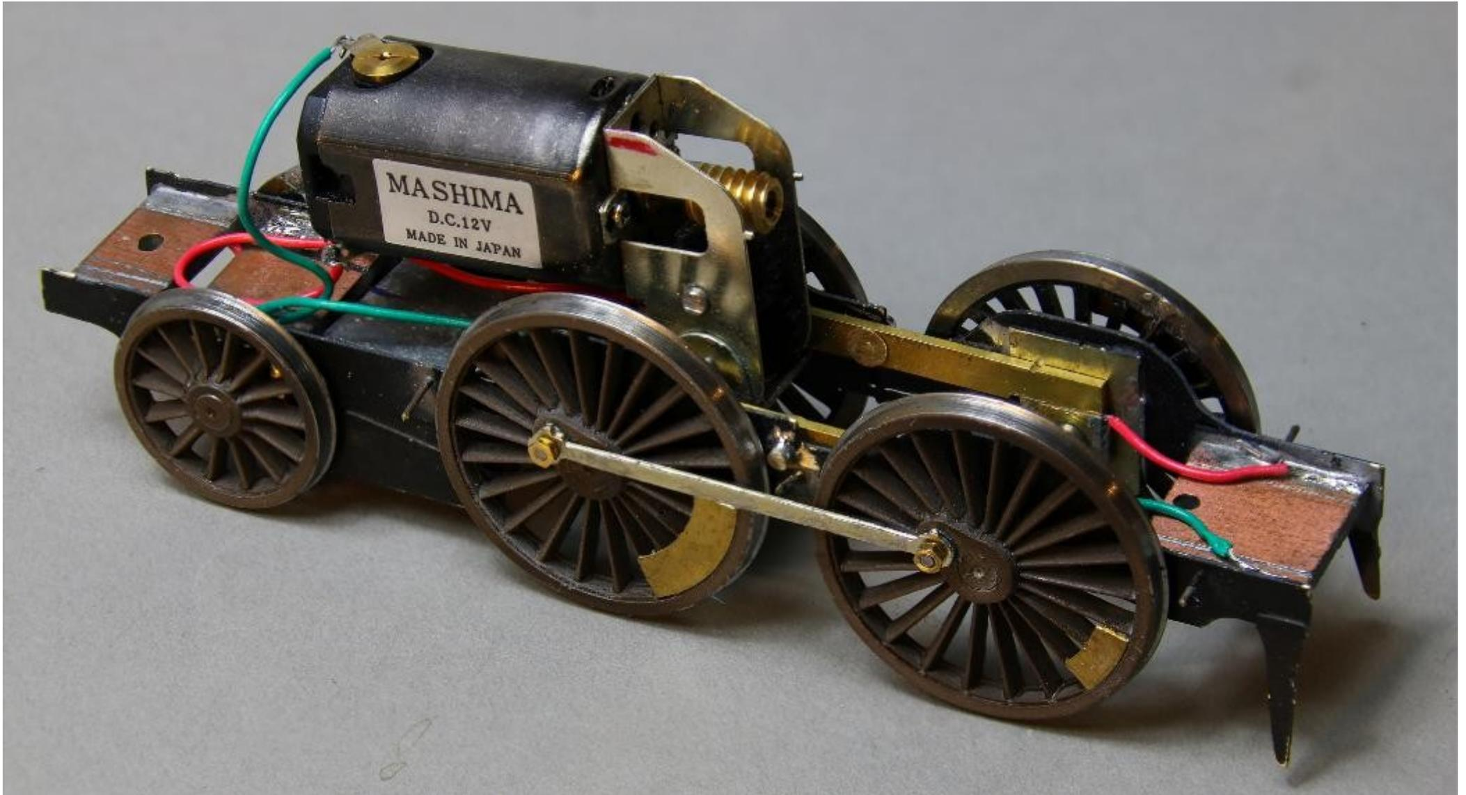
The tender chassis shows the side beams at the rear, whilst the leading axle runs freely, weighted down with about 20g of lead. The lead is glued to a strip of nickel-silver which pivots about the support for the side beams.
