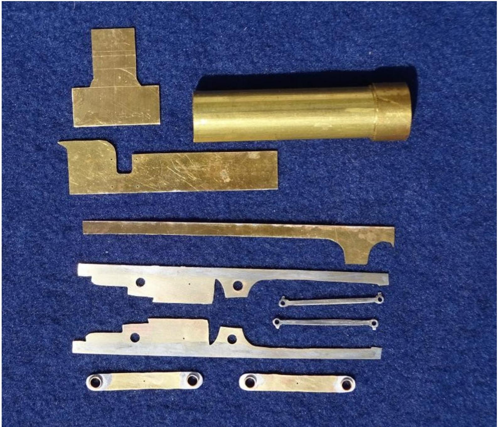
leading axle rocks on the 'roll axis' on a central pivot and the driving wheels are carried in a subframe that is pivoted at the mid point from both frames to provide movement in the 'pitch axis'. The compensation beams include the bearings for the driving axles so that there should be no variation in the distance between the crankpins as the driving wheels rise/fall. The arrangement is illustrated below.
