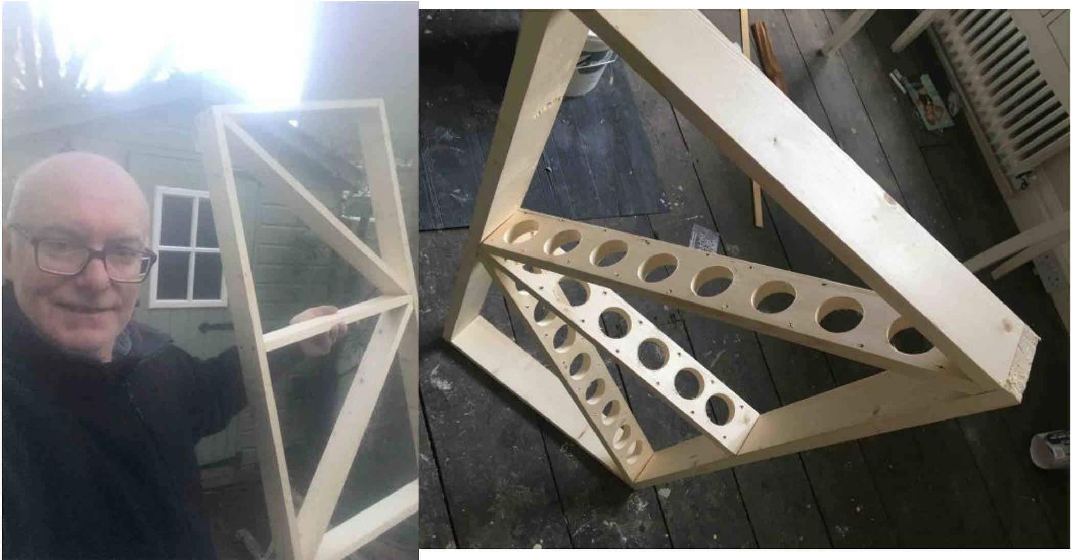
I therefore began by constructing the baseboard for this central section using a standard ply construction, hollowed out for lightness and future cable routes. Small isn't it!
