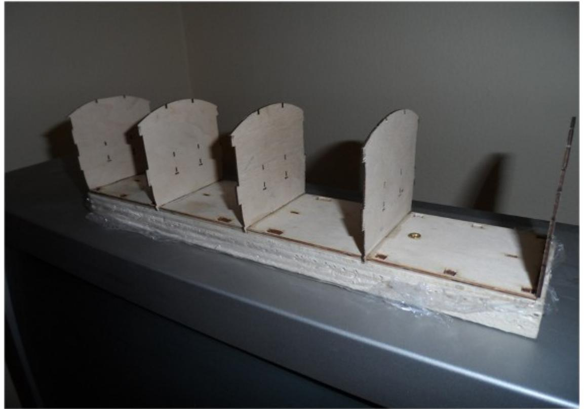
Next, the inner sides. Try them for a fit first, as the tabs on the side of the partitions should not only line up, but slide into the corresponding slots in the carriage sides. If all is well, apply glue to the sides of the partitions only down to the bottom of the middle tab. Again make sure the sides are lying completely flat and totally up against the partition sides.
