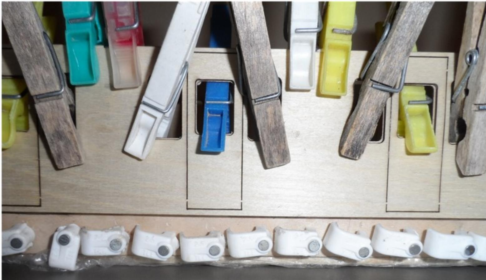
Again I use clothes pegs here to clamp as many surfaces together as possible. Leave to dry overnight, but check carefully for any loose sections. Re-glue and clamp as necessary. It is highly unlikely that every part will be glued up perfectly, but it is much more difficult to correct once the lower part has been clamped down as it causes any un-glued sections to bow out.
