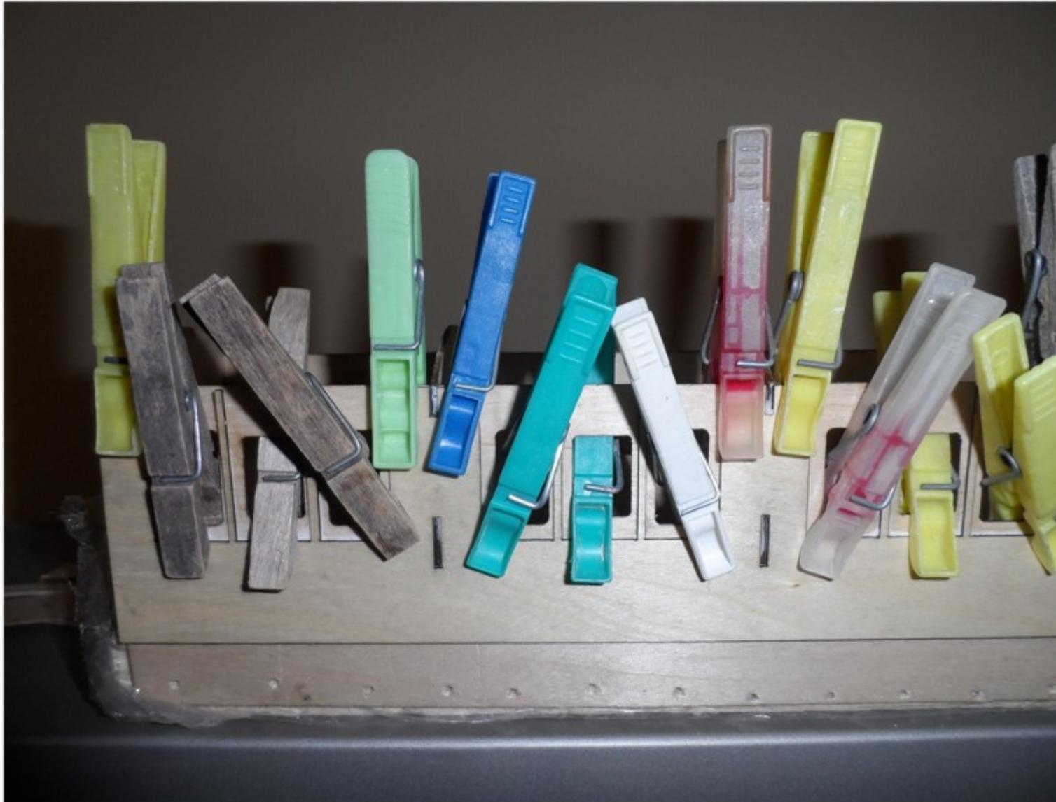
Once dry, remove the clothes pegs and check each fine extension to ensure they are well attached to the inner side. It is important as they are the sole attachment for the upper part of the outer side. If they are loose, the outer surface becomes slightly proud, and will flex in and out when touched. It is important to ensure that everything is well glued down. Apply copious quantities and then wipe off the excess.
