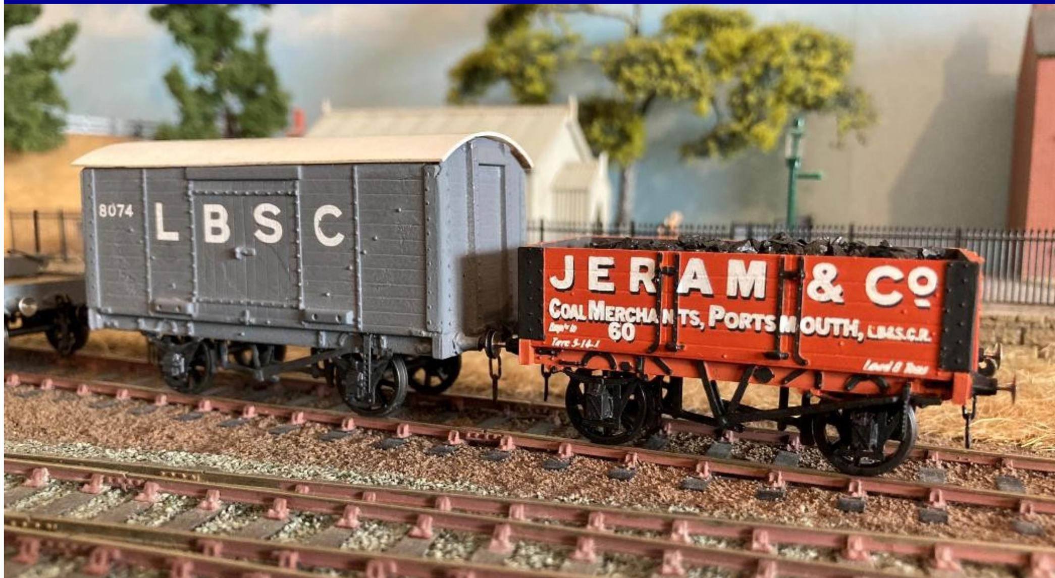
The covered van is from a Nucastr kit with Alan Gibson P4 wheels. I got it already assembled, but in need of some renovation and, although it is not compensated, it is squarely built and quite heavy, so track holding doesn't seem to be a issue. It is fitted with single V hanger single side brakes and a spare metal brake lever from a Hornby PO wagon.
