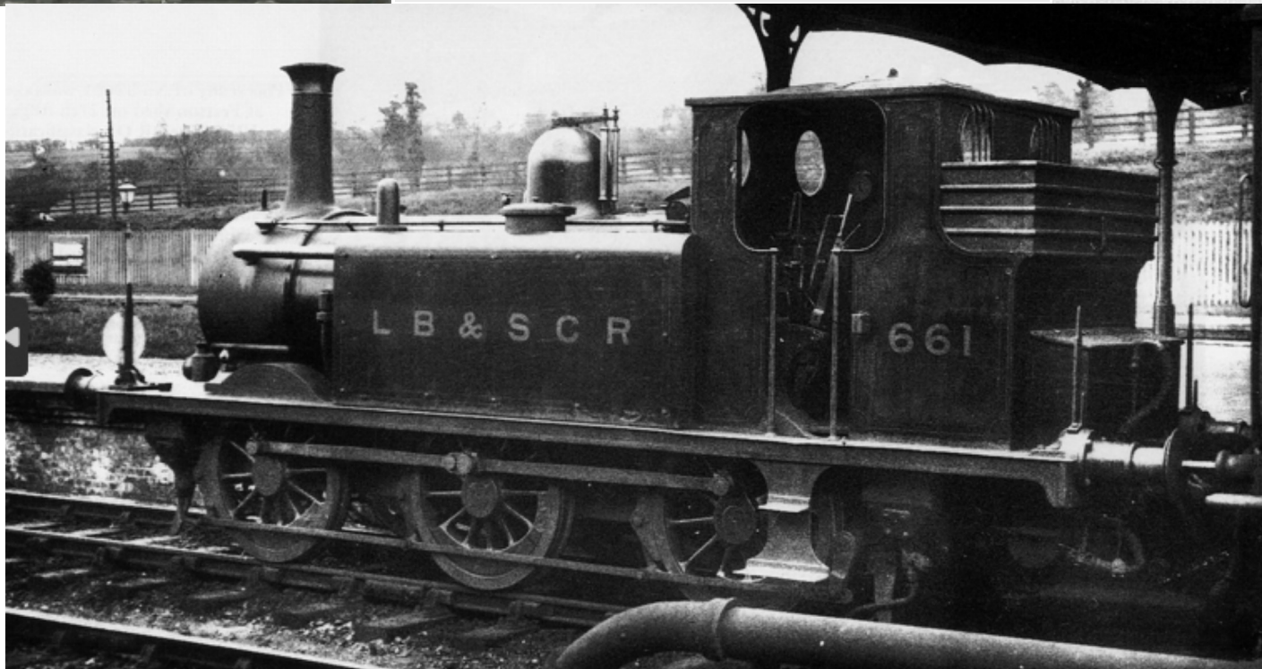
Below - A1X Terrier, as running 1913, showing the use of double height irons front and back
