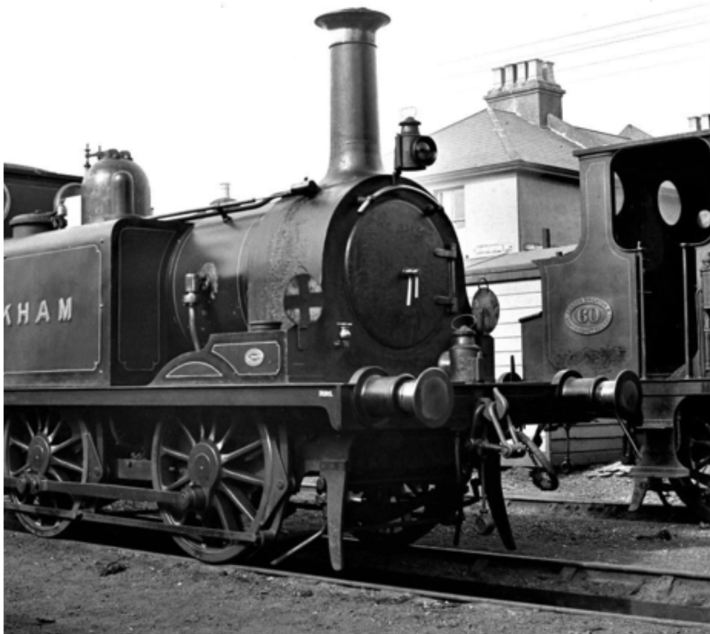
A1 Terriers - Left, as built with four irons and right, as running in 1918, still with four irons.
