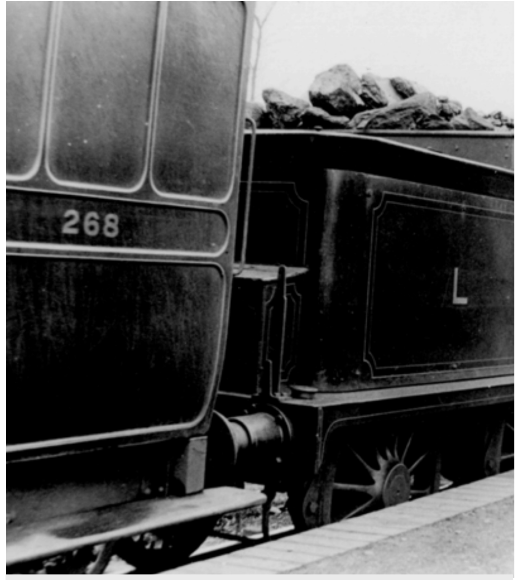
Rear of Stroudley tender, showing the use of double height irons.
