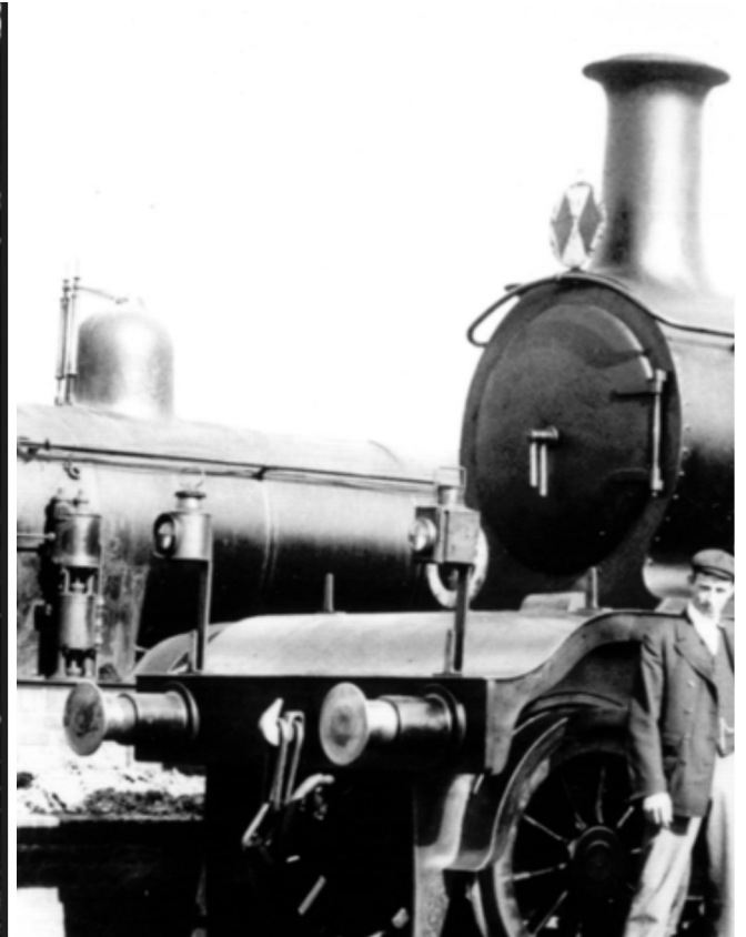
B2 4-4-0s. Left, as originally running with three irons on the upper level of the running plate. Centre, as finally running with two single and two double height irons at buffer beam level and a central one on the upper level of the running plate. Right, incorrectly running with all eight irons!
