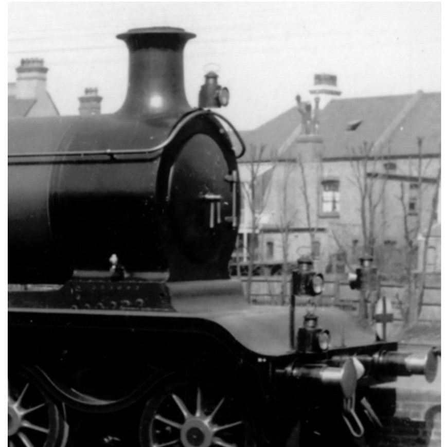
B4, displaying a one board code, but with four lamps (one reversed) 'resting'.
