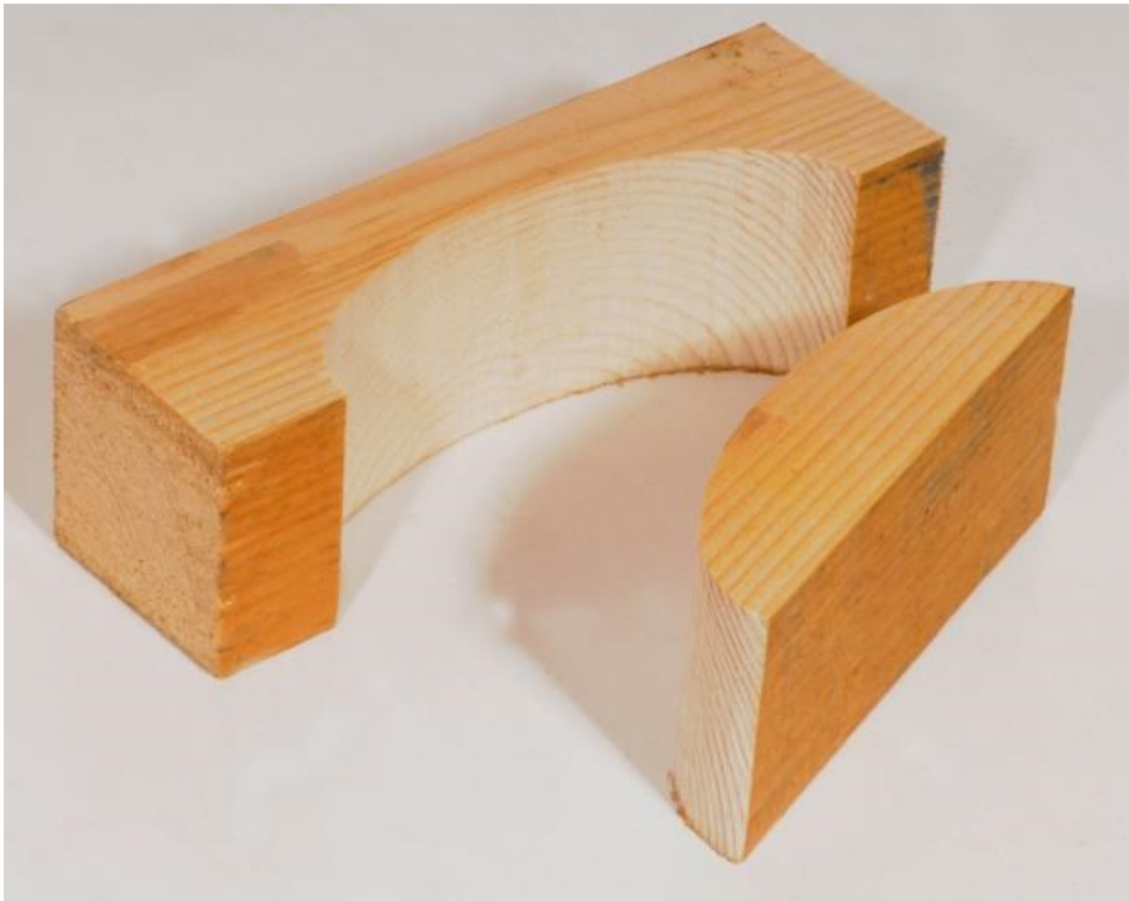
Picture 112 Former for laminating, cut from a solid block of timber.
