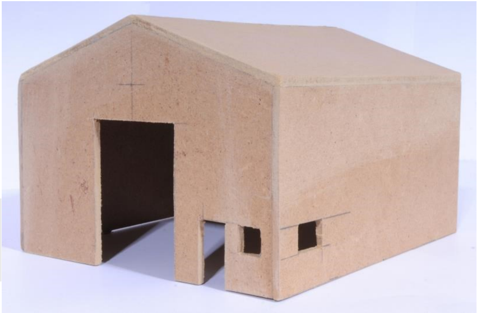
Picture 111 Structure to form the shell of a building made from 6mm MDF.
