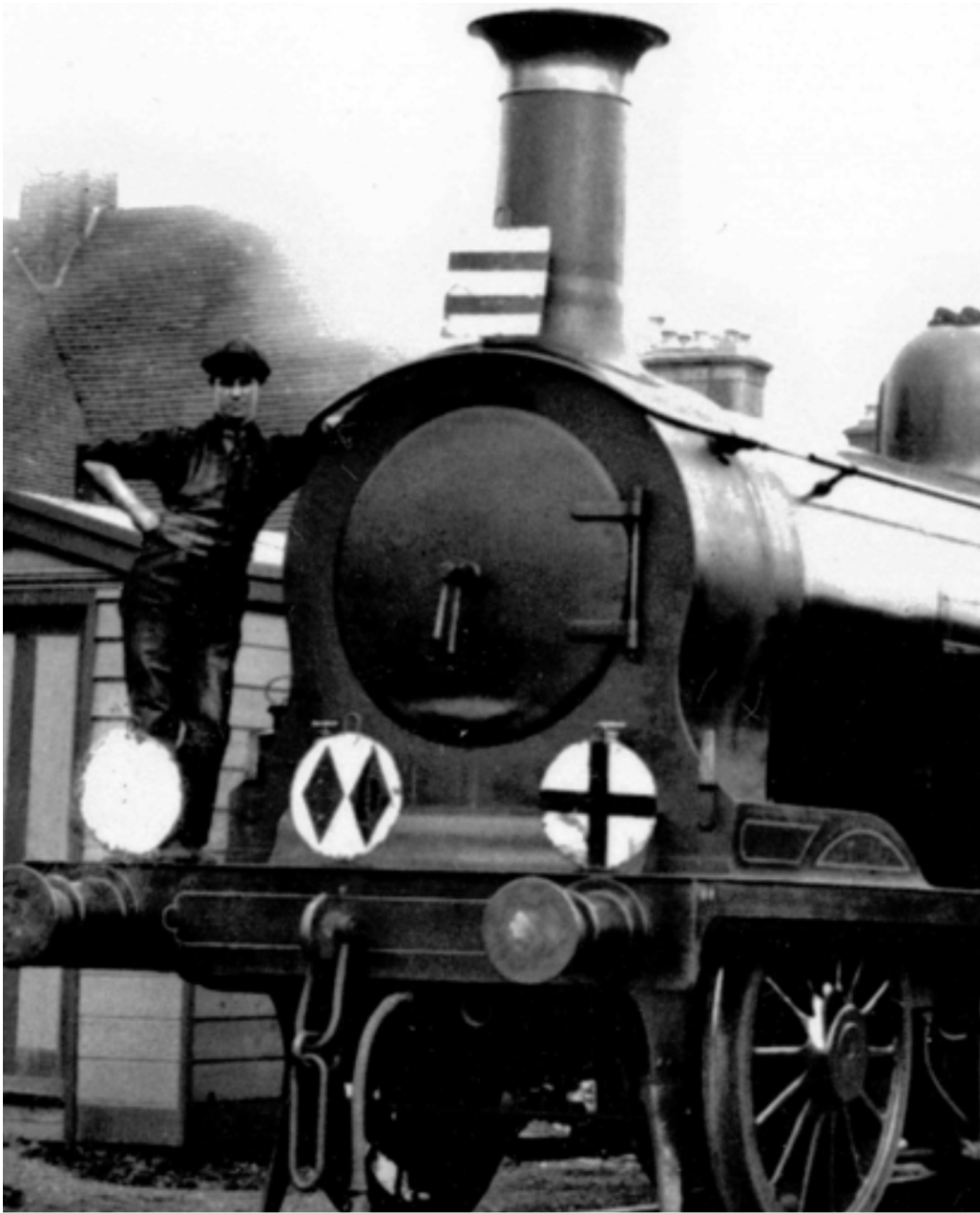
Stroudley G Singles, with new irons fixed on bufferbeam, showing how the higher position is hidden.
