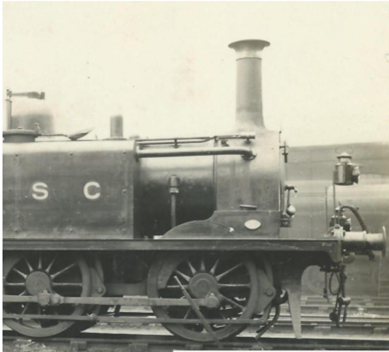
Left - A1 Terrier, as running c.1915, showing the use of double height irons.
