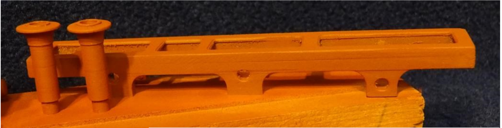
The printed frames and chimneys, after a coat of Holts red primer.
