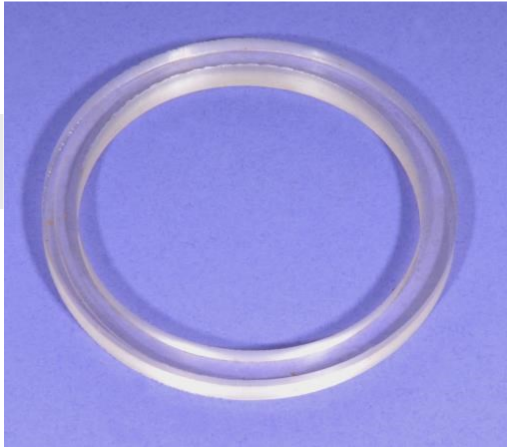
Picture 118 Acrylic ring turned in the lathe.
