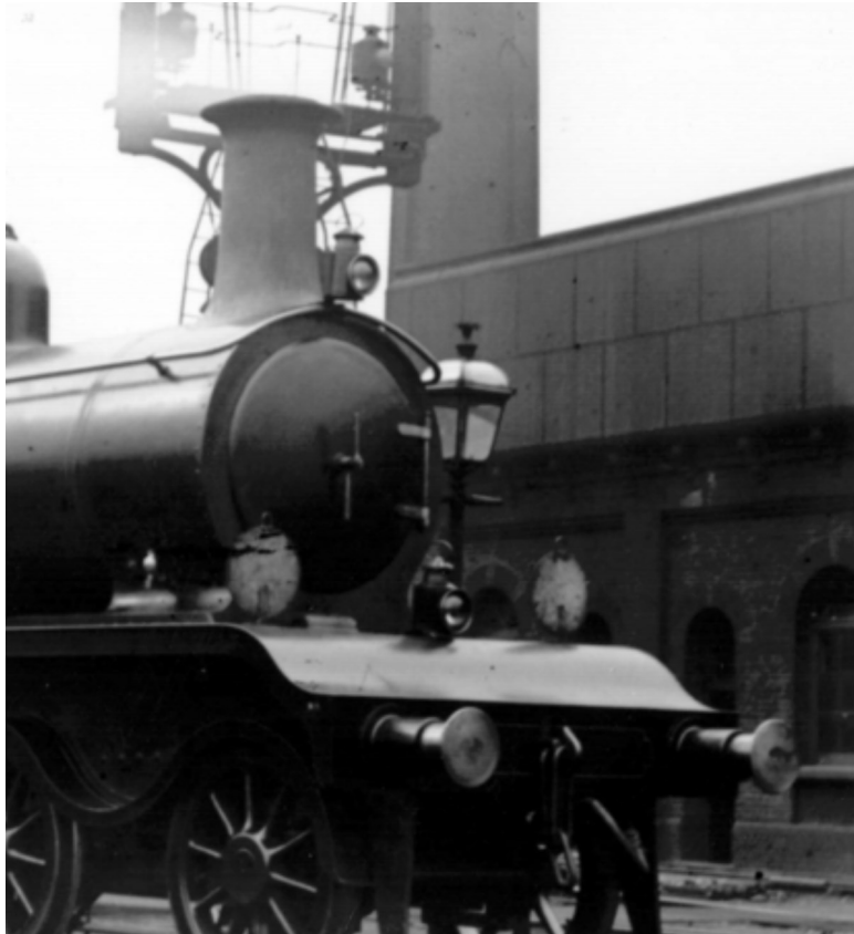
B2 4-4-0s. Left, as originally running with three irons on the upper level of the running plate. Centre, as finally running with two single and two double height irons at buffer beam level and a central one on the upper level of the running plate. Right, incorrectly running with all eight irons!
