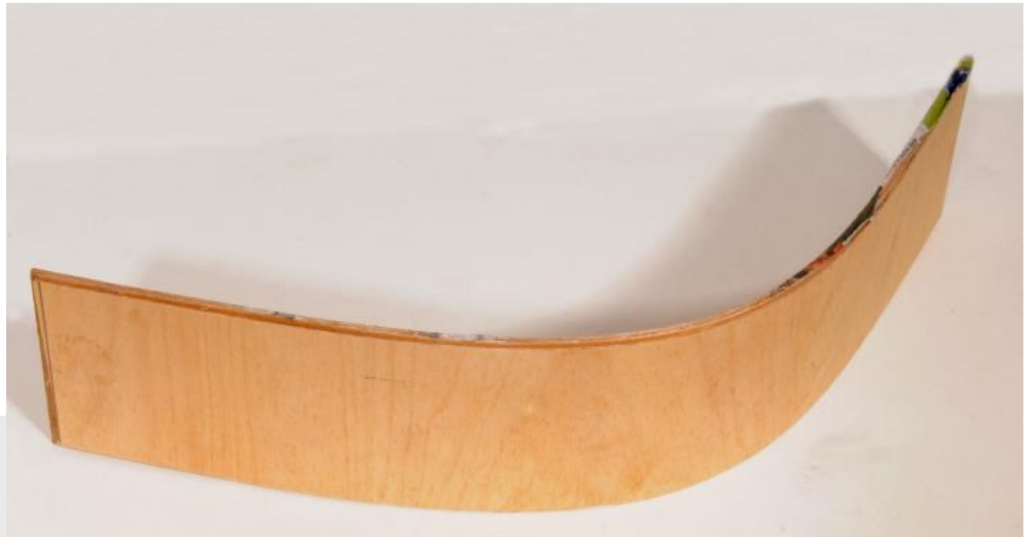
Picture 115 Finished laminated shape. ready for cleaning up.
